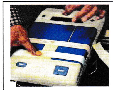
Sealing with Outer Paper Strip Seal (ABCD Seal)
